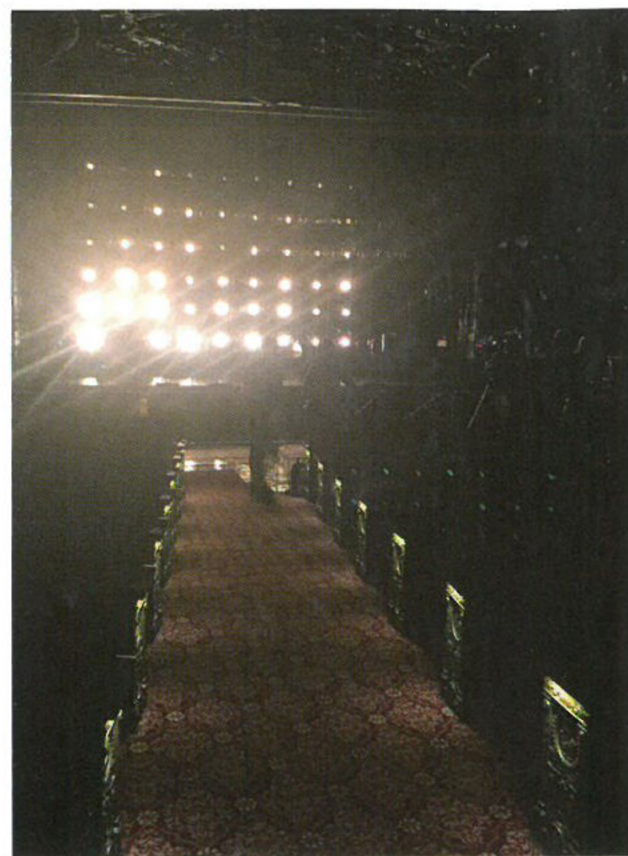
For a funkadelic concert by the fictional singer Hannibal (Daniel J. Watts, top left), Morano had gaffer Ben Noble rig 64 500-watt Par cans on a black pipe grid. The Pars, which were run through a dimmer system, created a wall of light behind the performers.
